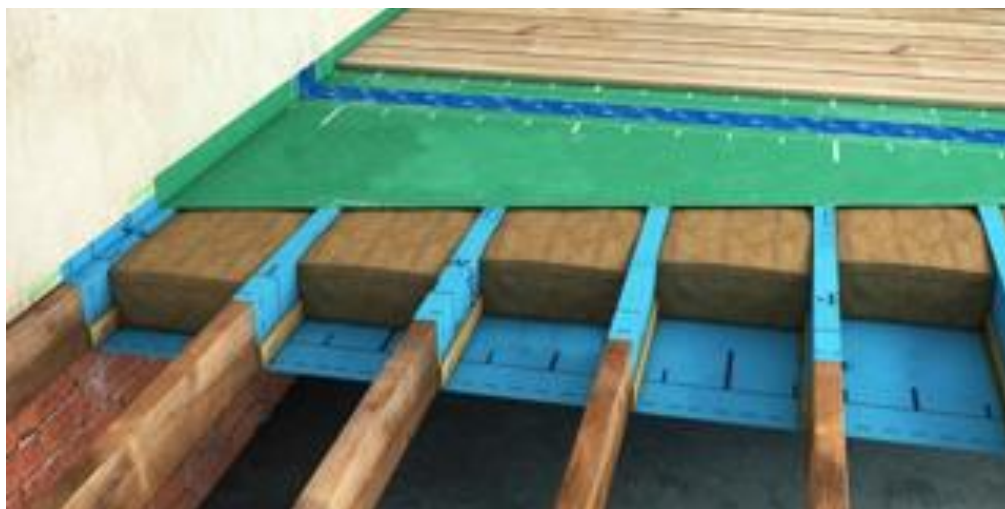
Figure 45 Example of an airtight, vapour permeable membrane (blue) under the insulation (hemp insulation) and the vapour control layer (green) above the insulation.
