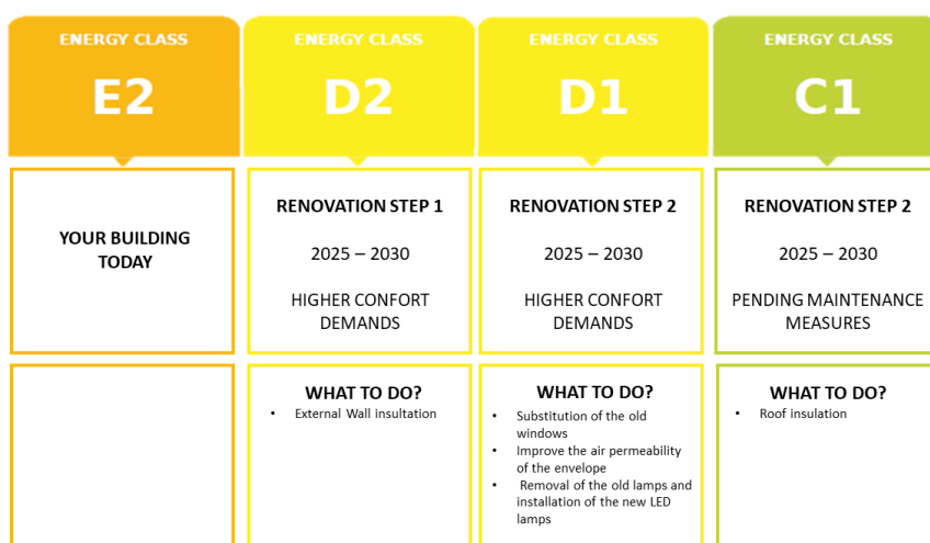
Figure 7 Example of a renovation roadmap developed for an 1877 solid stone wall building.
