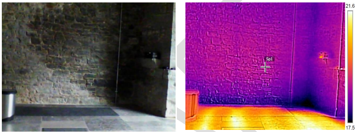
Figure 12 Thermal image showing thermal gaps at junctions.
