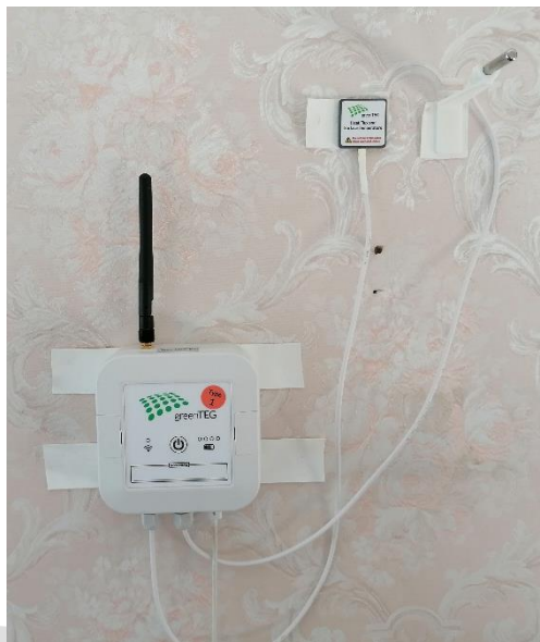
Figure 15 In-situ U-value measurement kit installed on the internal face of a wall.
